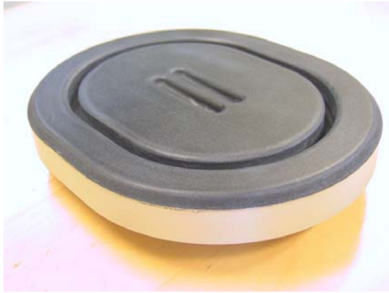
Figure 4. An example of sensor head with measuring slots and tightening ring for sucking of leakage air.
